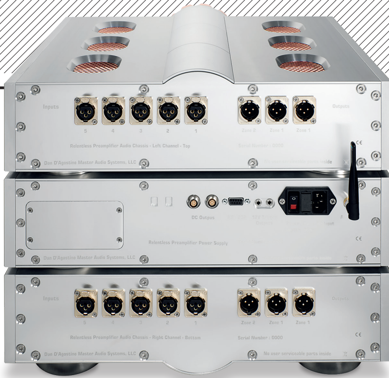
ABOVE: All switching/phase invert and other logic controls are fed alongside PSU rails through connectors in the top plate and front left foot of the centre unit. The top (left channel) and bottom (right channel) preamps offer five balanced inputs, two Zone 1 and one Zone 2 balanced outputs. Remote is via Bluetooth control
